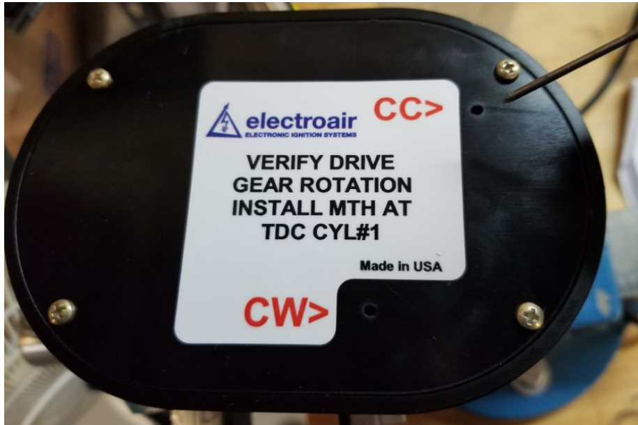
Figure 10: Installation of MTH Alignment Pin
