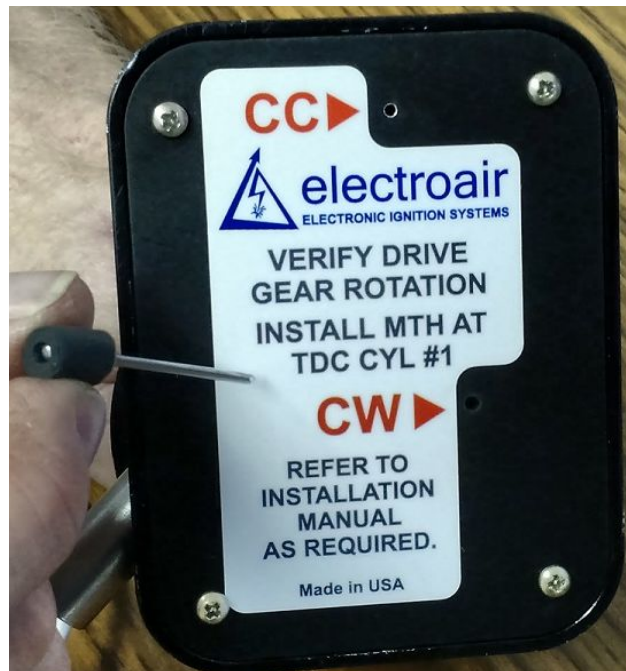
Figure 7: Installation of MTH Alignment Pin
